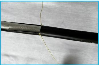
Once the armour has been removed, move on to removing the inner sheath and exposing the fibre.
