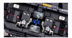
Faster fibre transportation time The 45S's wind protector and fibre clamps are linked: when the wind protector opens, the fibre clamps open. The fibre retention clamps gently hold the spliced fibres in position to prevent risk of breakage. These mechanisms provide easy fibre handling and faster transfer to the heater.
